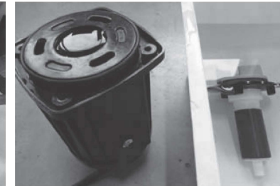
5. Put pump body in a vertical position and fill with a mild lime scale remover (like cleaning vinegar). Immerse rotor in a plastic bowl/container filled with the same lime scale remover and leave both for 24 hours. After 24h rinse off with water and re-assemble pump.
